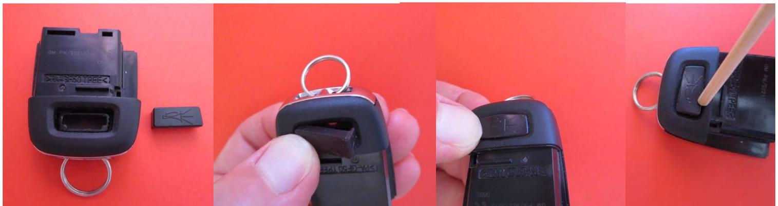
Next you press new Black panic button in using your thumb and finger nails. If it is bit hard to push with finger nails you can use blunt side of skewer to press on button edges.
