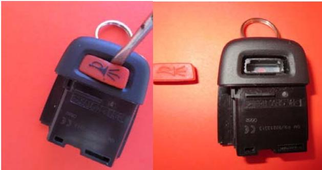
Depending on the condition of your button you can remove it simply by lifting up with flat screwdriver or with Stanley knife.
