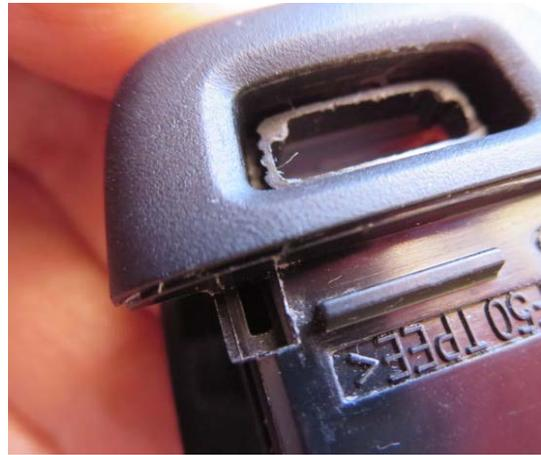
Before you start fitting new button in, make sure button cut out is clean from old rubber remnants.
